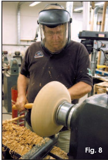
Bill took his turn on the lathe by rough-turning the inside.
